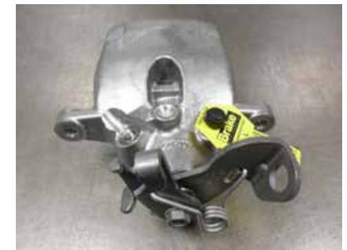
CA3090 (BHS1206/7) - Vented Aluminium Piston = 41 mm Pad Gap 72 mm Slider pitch = 134 mm Cast codes 17/0901 & 17/0902 Mechanically activated h/brake
