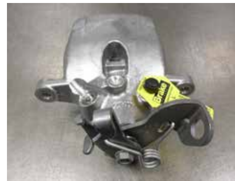
CA3090 (BHS1206/7) - Vented Aluminium Piston = 41 mm Pad Gap 72 mm Slider pitch = 134 mm Cast codes 17/0901 & 17/0902 Mechanically activated h/brake
