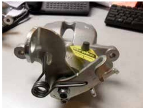
CA2957/R (BHS1202/3) - Solid Aluminium Piston = 41 mm Pad Gap = 61mm Slider pitch = 134 mm Cast codes 16/6101 & 16/6102 Electrically activated h/brake
