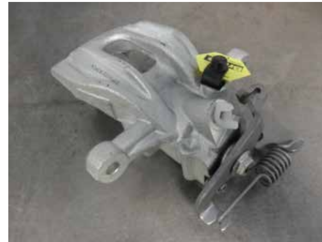
CA2620/R Bosch Cast Iron with 38 mm piston Slider pitch = 127mm Cast code = 0204Y01681 (LH)
