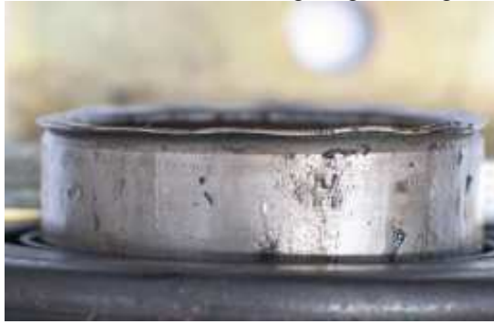
Over-stroke retaining ring damage
