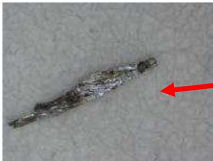
Aluminum swarf causing leakage from gear side
