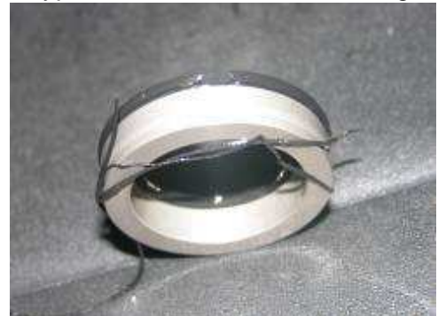
Typical Over-stroke seal damage
